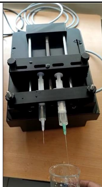
Figure 10: Multi Syringe Pump set up for purging fluids in micro-channels.
